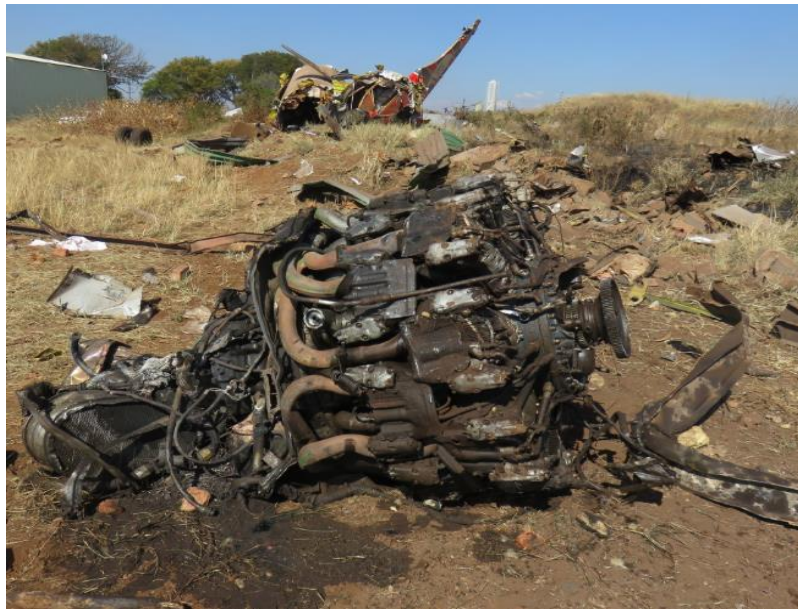
Figure 22: The left-hand engine as it came to rest.
