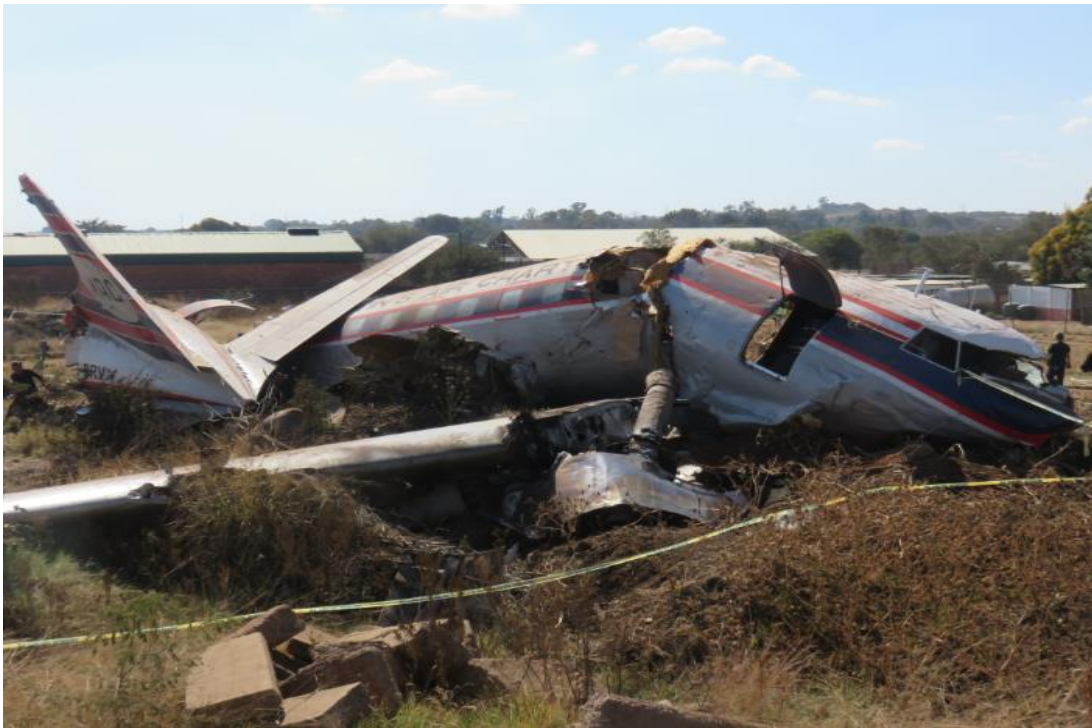
Figure 21: The aft section of the aircraft had separated from the fuselage.
