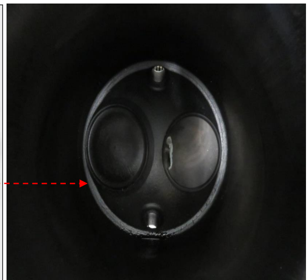
Figures 35/36: On the left is the 18 double-row, air-cooled Pratt and Whitney R-2800 radial engine and on the right is an image of the No 7 cylinder combustion chamber, showing a fractured exhaust valve head.
