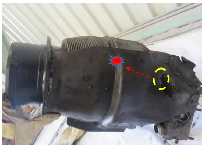
Figure 39: An image of the No 7 cylinder showing the fire damage on the exterior through the cooling fins and the plate.
