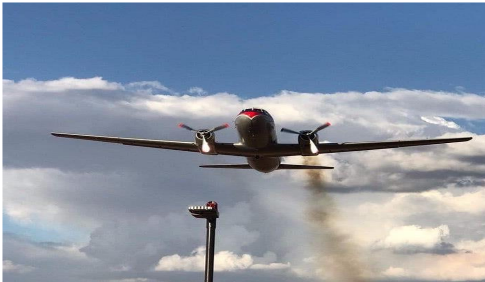
Figure 1: The aircraft with black smoke trailing from the left engine/No 1 engine.
